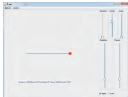
Figure 2: Screenshot of the program, which presented the micro-gestures to be performed (the example shows the sweeping gesture). The right index finger should follow the position of the red dot moving along the line. With the help of the sliders on the right hand side the gesture parameters could be adapted.
